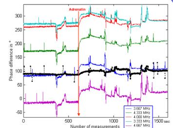
Injection of suprenarine at sample point 600. The pressure changes as well as changes in consistency and density of the cell substances could be measured directly.
