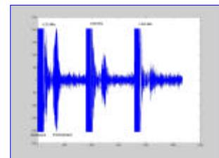
Example of a trace recorded by the receiver. It consists of the three transmission impulses (4.33 MHz, 4.66 MHz and 5.0 MHz) and the respective echoes. The amplitude of the echo is reduced due to the minimal bandwidth of the U/S sensor and the decrease in signal strength due to the tissue when using higher frequencies.
