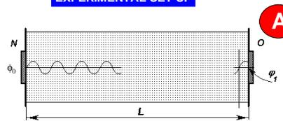
The general idea of measuring method is presented for the simplest case, i.e., for homogenous and isotropic media. In this case phase velocity of an acoustic wave depends on both the medium elasticity  $K$  and the density  $\rho$  in accordance with equation:
